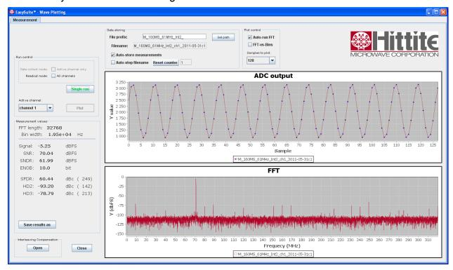
The Wave Plotting window contains the run control settings in the upper left corner. Data storing settings are located at the top. In the bottom portion of the window are two charts, one for the transient output and one for the FFT plot.
